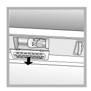
Access the light bulb by removing the cover as indicated in the diagram. Replace it with a similar light bulb within the power range indicated on the cover (10W).
